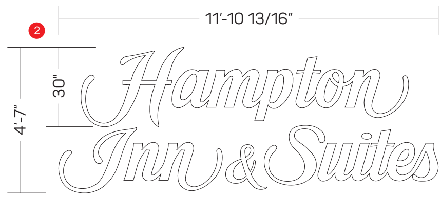
CHANNEL LETTER DETAIL SCALE: 1/4" = 1'-0"
