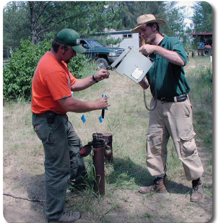
Bemidji Crude-Oil Research Project; measuring crude-oil thicknesses during the aquifer test.
