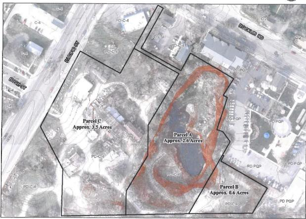
**Contour map.** Please note that the proposed parcel boundary around Parcel A closely follows the perimeter of the quarry. On an aerial such as that on page 13, the south end of the quarry pit looks flat, however, it is a steeply graded entrance access to the bottom of the quarry pit. See photos on page 12.
