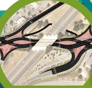
Concept 2: Diverging Diamond Interchange with Separate Ped/ Bike Undercrossing
